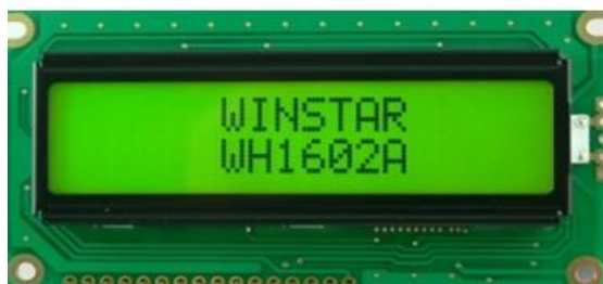
Slika 6: LCD zaslon Winstar WH1602A (Vir: www.winstar.com.tw )
