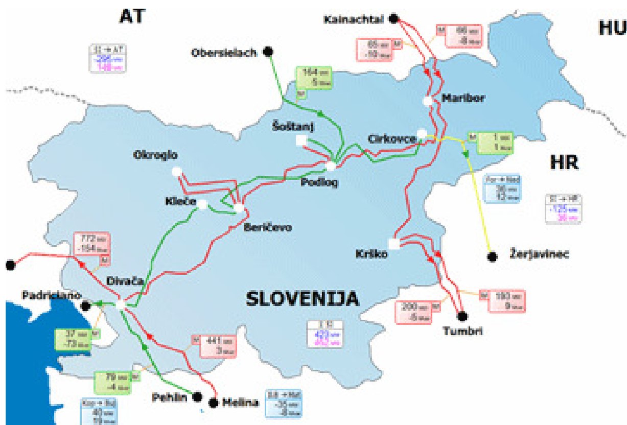
Fig 4-1. Slovenian high voltage transmission network. (ELES, 2010)
