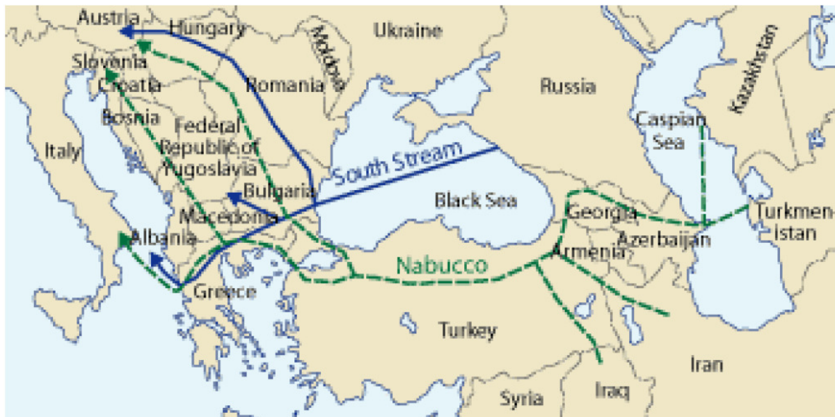
Figure 3-12: Southern corridor of supply way with natural gas – Nabucco and South stream /23/
